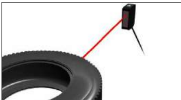
Detection of tire passage
