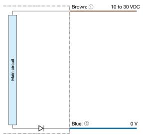
\*For the universal voltage type, add 24 to 240 VAC / 24 to 240 VDC to the brown wire and blue wire. (No polarity)
