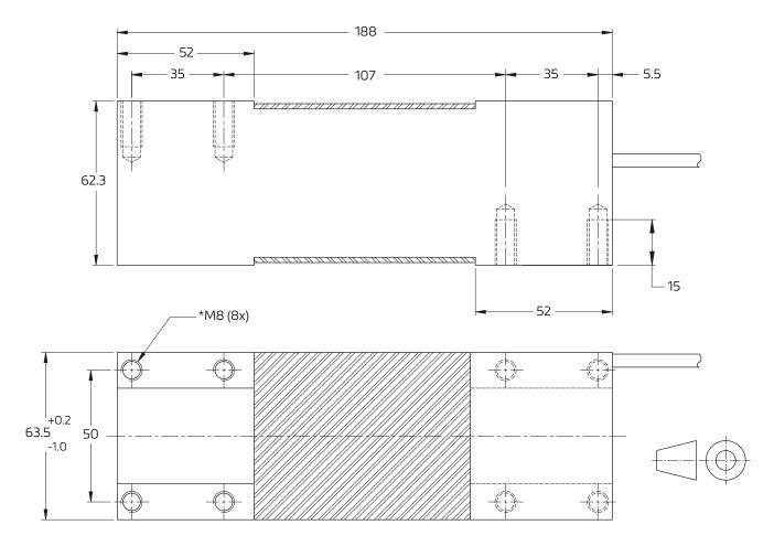
Mounting bolts M8 8.8; torque 25 Nm. Torque value assumes oiled threads.
