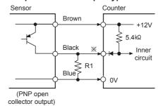
※In case of PNP open collector output type sensor, please connect lower than 470Ω of R1 to input terminal before using. (A) Photoelectric Sensors
