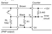
※Please set R1 value to make the composed resistance of RL + R1 as Max. 470kΩ is an impedance for short-circuit.
