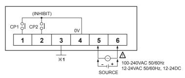
X1: It can be selected RESET or sensor power (+12VDC 50mA) by internal PIN operation. (Refer to J-40)
