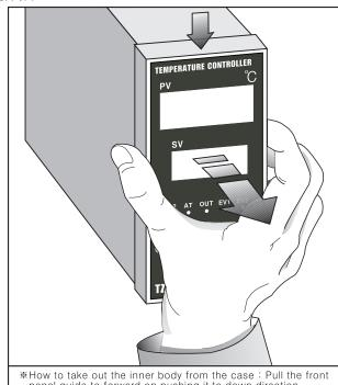
panel guide to forward on pushing it to down direction.
