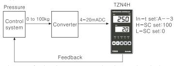
\*In case of using the converter mode, please select the inner switching pin according to the chart in "Selection switch for Input sensor/Voltage/Current"
