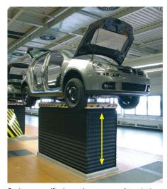
Customer-specific draw-wire sensors as important OEM component: Draw-wire sensors monitor the height of lifting platforms on automobile production lines.
