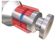
To monitor the clamping position of tools, a VIP sensor is integrated into the release device and directly measures the clamping stroke of the drawbar.
