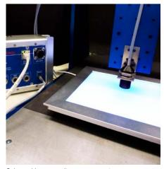
Color and homogeneity measurements of LED/lighting panel.
