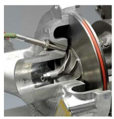
Rotational speed measurement of turbochargers
