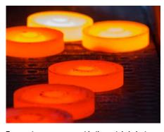
**Temperature measurement in the metals industry**Temperature monitoring in the cooling processes of forged parts using the CTLaser M1
