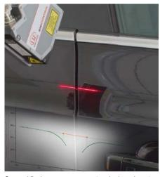
Gap and flushness measurement on bodywork parts
