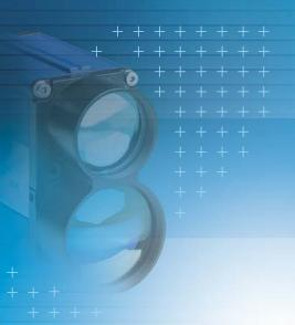
Optoelectronic optoNCDT ILR sensors are designed for non-contact distance and displacement measurements with large measuring ranges. The 118x series is based on the phase comparison principle, where modulated laser light is permanently transmitted to the object. The receiver compares the phase shift of the transmitted signal with the received signal, enabling the distance to be precisely calculated.
