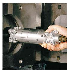
Inspection of inner diameter in extruder bores
