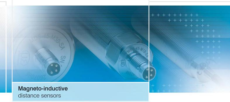
Magneto-inductive sensors measure displacement, distance or position of a defined magnetic target. The measuring range is 45 mm as standard, but can be adjusted from 20 mm to 55 mm by changing the magnet. This physical measuring principle means the output signal is linear (2 - 10 V and 4 - 20 mA) and is independent of the measuring range.
