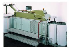
**Example: machine monitoring**Eddy current sensors monitor the fluctuating thickness of yarns in textile machines.
